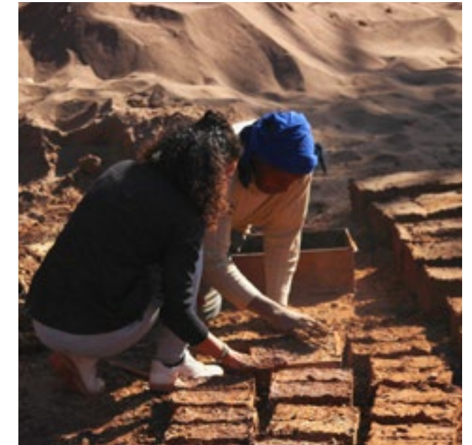
Tamping of the mud and straw mix into a wooden brick mould
